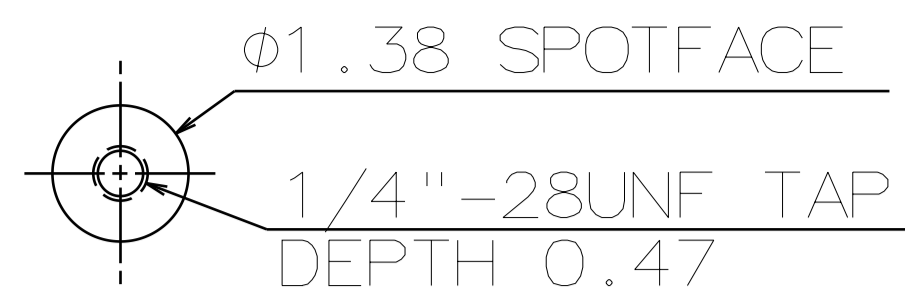
DETAIL A (PROVISION FOR VIBRATION SENSOR)
